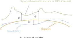
h=ellipsoid height H=orthometric height N=geoid height
