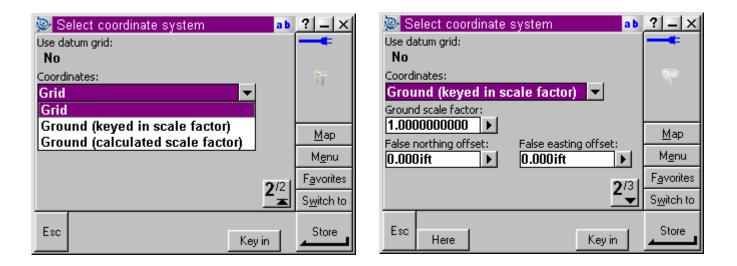
All Survey Data will be collected using Grid Coordinates. For final Ground Coordinate data submission, data will be converted to ground per "Design to Construction Automation" Manual beginning on page 19
