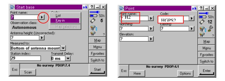
**NOTE:** When Using False Coordinates, Such as "You Are Here" **you must put an "H" in front of the point number, and code**. Ie. Point Name (H2), Code (HGPS2).
